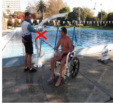
Actuator – Never push on actuator to rotate the Lifting arm. This will damage lifting mechanism
